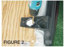
2.) Cut out "pentagon" shaped hole templates from side of instruction sheet and place on bottom side of handles as shown. (see figure 1) Drill 3/8" hole as marked by template. (see figure 2) Enlarge existing stock hole to 3/8" to aid in installation. (see figure 3)
